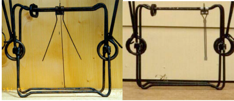
Figure 2. Standard V-trigger conibear trap and modified conibear trap.
